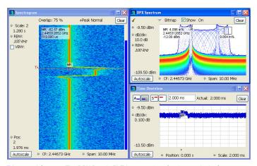
Trigger and Capture: The DPX Density™ Trigger monitors for changes in the frequency domain, and captures any violations into memory. The spectrogram display (left panel) shows frequency and amplitude changing over time. By selecting the point in time in the spectrogram where the spectrum violation triggered the DPX Density™ Trigger, the frequency domain view (right panel) automatically updates to show the detailed spectrum view at that precise moment in time.
